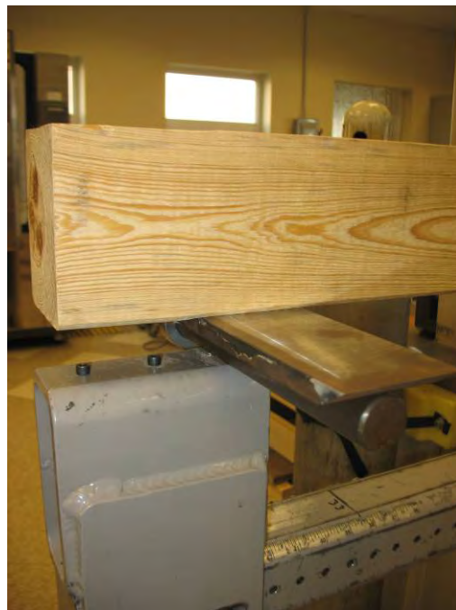
Photo No. 2 Typical Specimen End Support Detail
