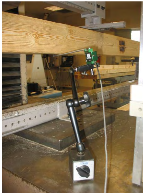
Photo No. 4 Deflection Measurement Apparatus
