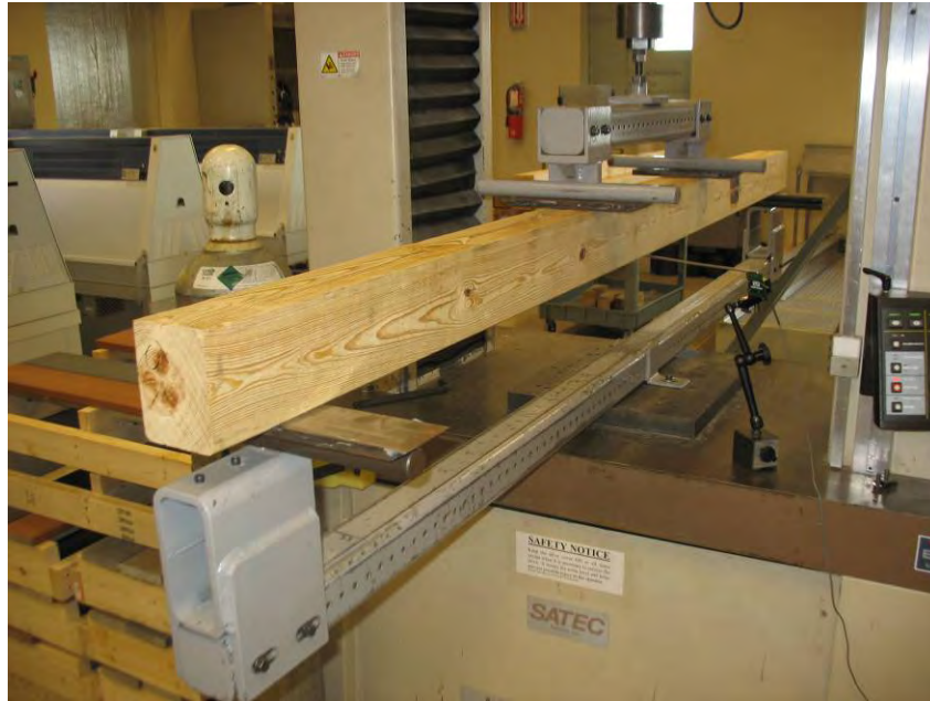
Photo No. 1 Flexural Evaluation Test Setup
