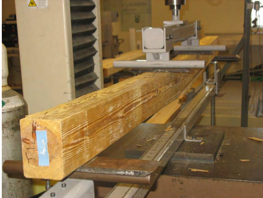
Photo No. 9 TimberSIL Test Series Specimen at Ultimate Failure Condition
