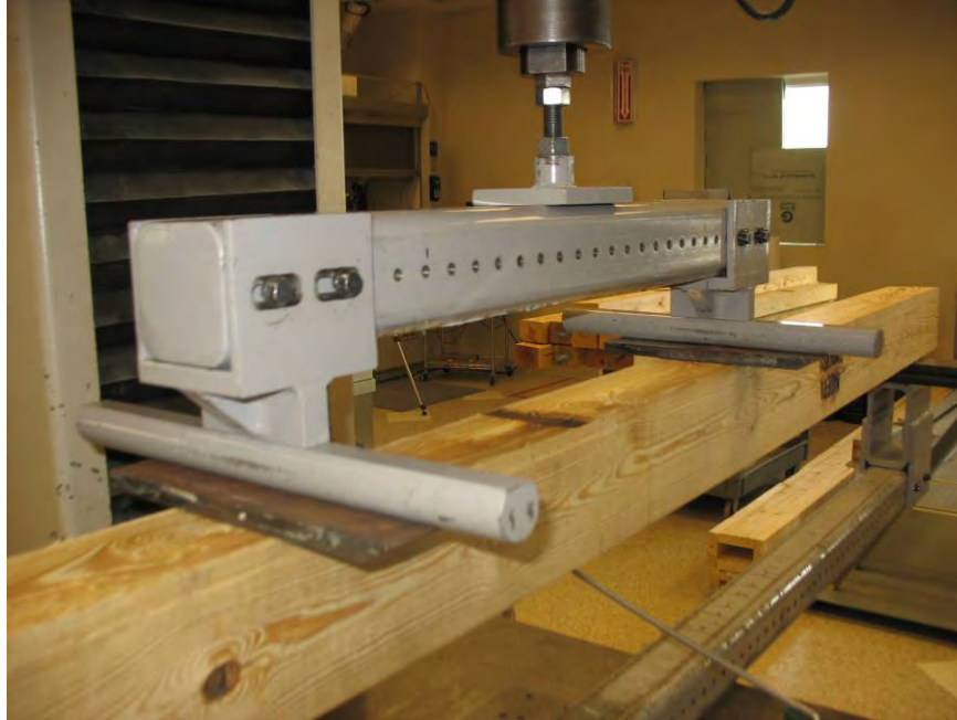
Photo No. 3 Typical Specimen Loading Detail
